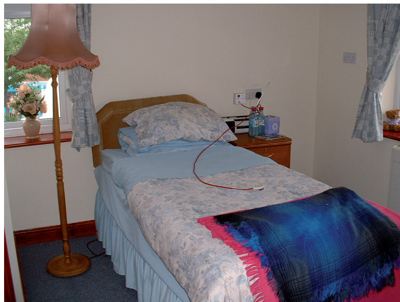
Figure 1: Carers can be alerted if alarm-cord extensions are used
